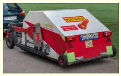
The Tiresonic Mk.3 trailer for tyre/road noise measurement
