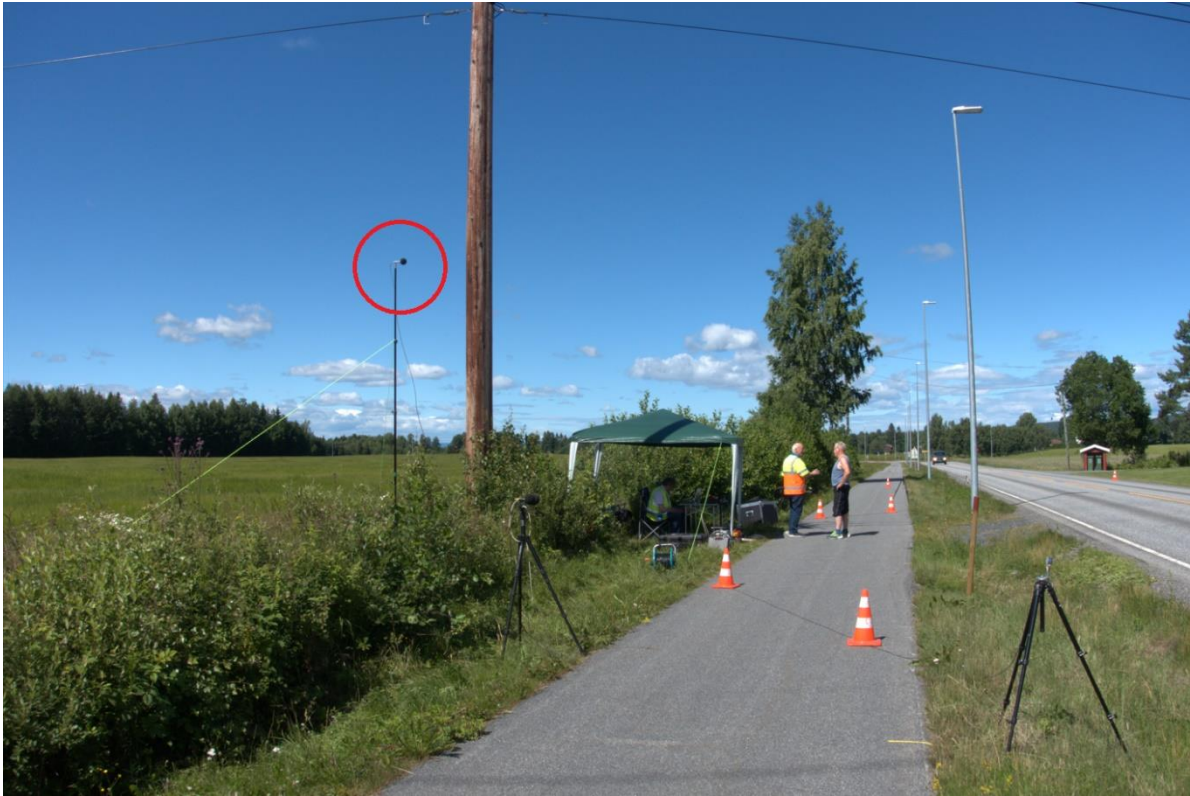
Figure 50. Location of the measurement microphone in the road surroundings in Sørum (SMA16 surface)
