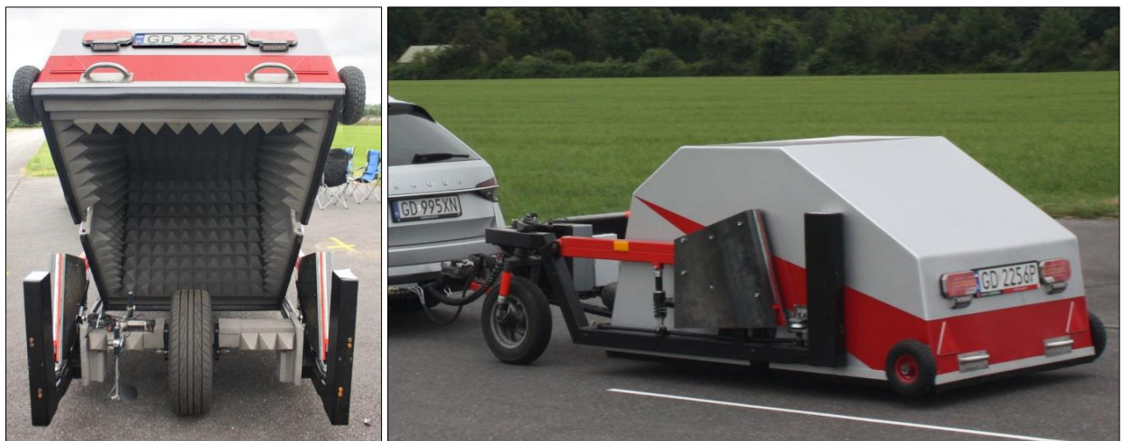
Figure 4. The GUT CPX trailer, Tiresonic Mk5
