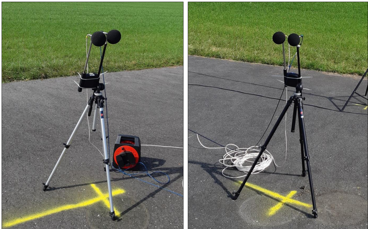
Figure 1. The position of the microphones (left: GUT's and right: SINTEF's) on both sides of the test track
