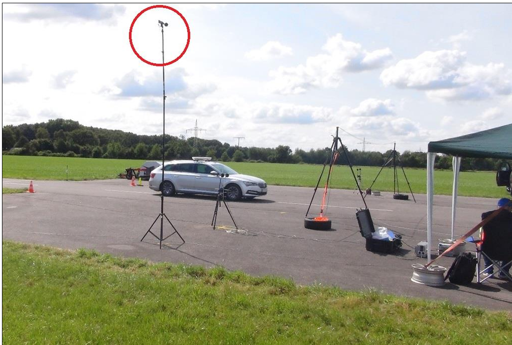
Figure 22. View of the location of the measurement microphone with sound level meter
