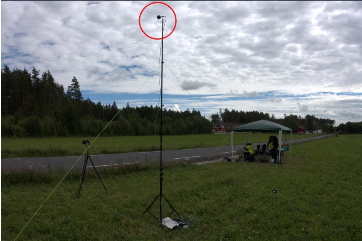
Figure 49. Location of the measurement microphone in the road surroundings in Skjeberg (Ma11 surface)
