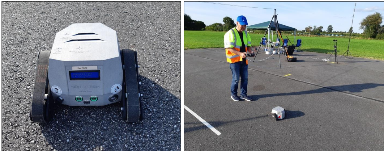
Figure 2. Surface texture drone (left) and conduction of measurements (right)
