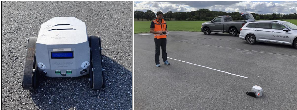
Figure 21. Surface texture drone (left) and conduction measurements (right)
