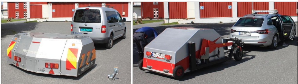
Fig.7 CPX trailers: Norwegian (left) and Polish (right)
