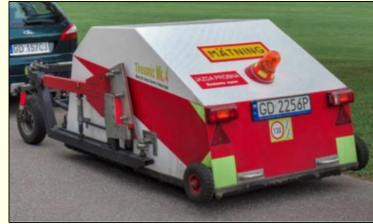
The Tiresonic Mk.3 trailer for tyre/road noise measurement
