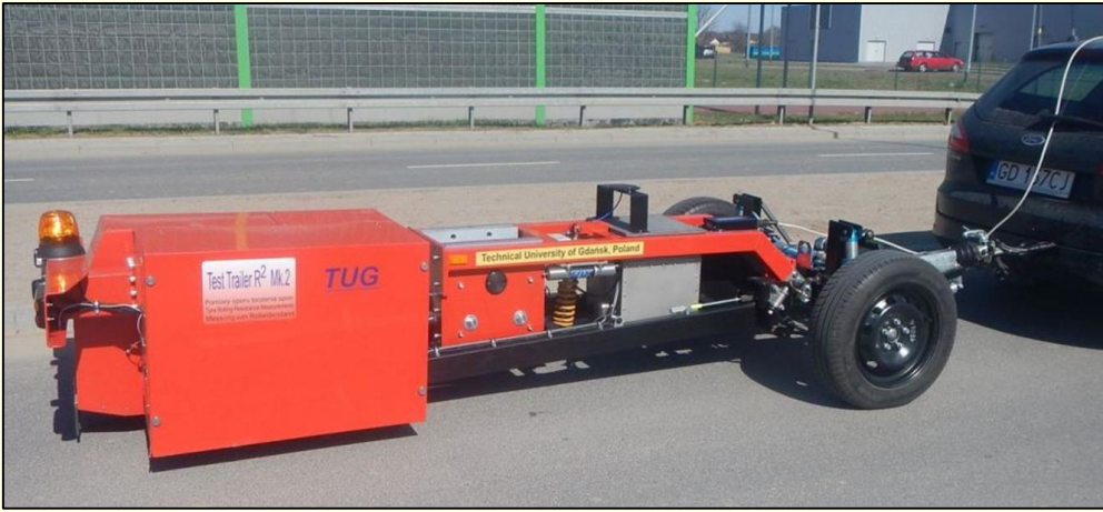
The rolling resistance trailer R2Mk.2
