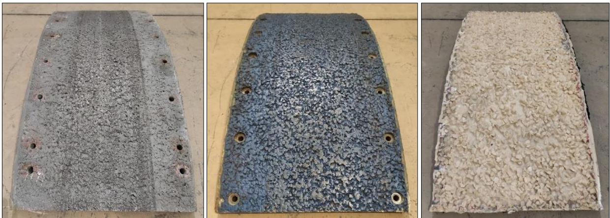
Fig. 2. Replica road surfaces used in noise measurements (from left: ISO, SMA8, APS)
