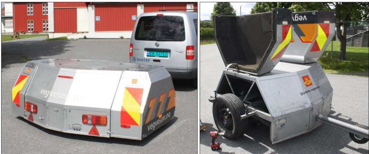
Figure 2. Norwegian CPX trailer
