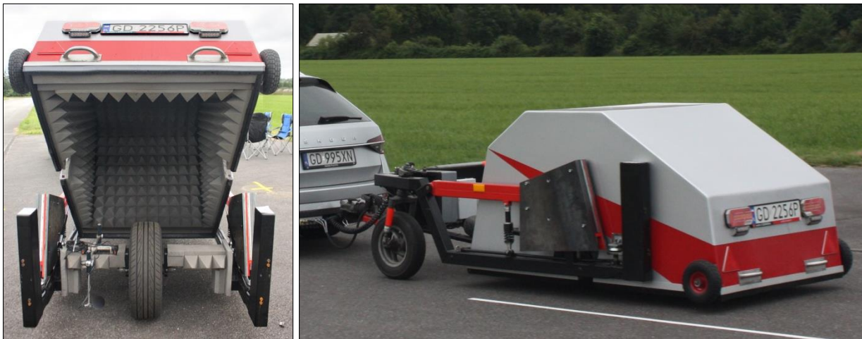
Figure 1. Polish CPX trailer, Tiresonic Mk5
